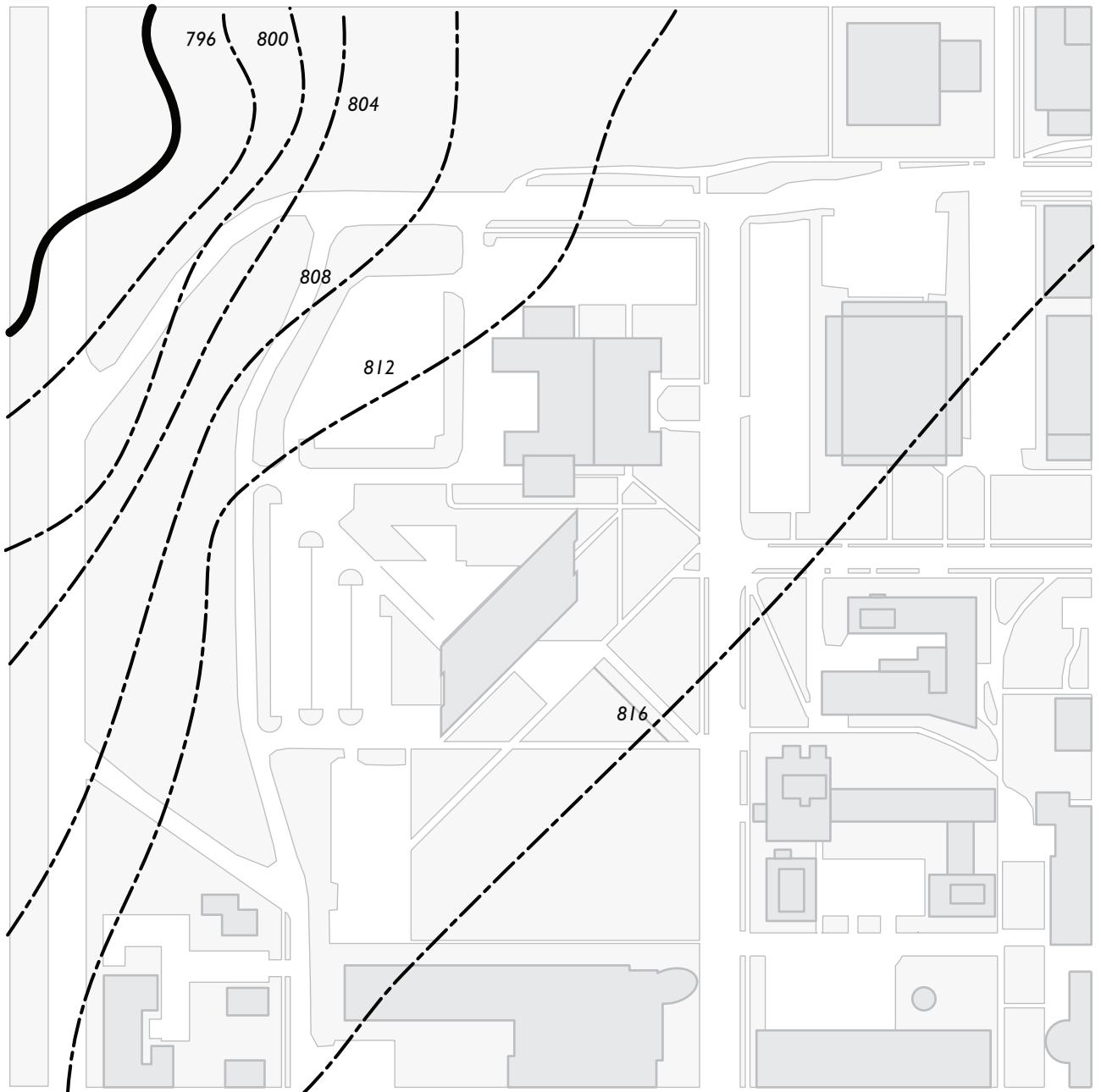
Figure 1.2.3. Understanding the geography of the site includes a full topographical survey (typically provided) by the client that can be interpreted to show steep slopes, runoff areas, and physical orientation.
