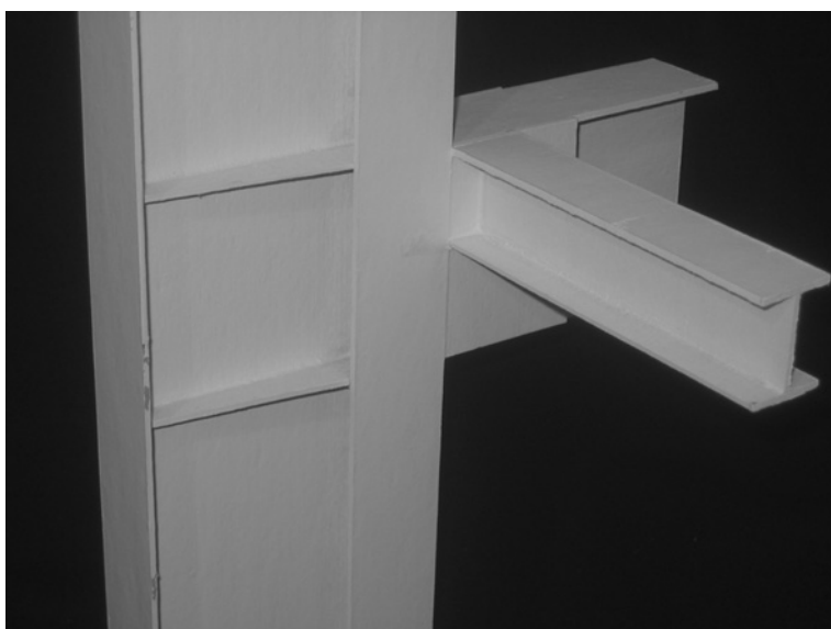
Figure 4.8.13. Model of a typical moment connection at Inland Steel's perimeter. Additional steel plates have been added to the column to carry the geometry of the beam through, creating a 'moment box.' This provides the stiffness to keep the building frame from twisting unevenly due to the asymmetrical bracing in the core. (Model by Doug Conroy and Asa Westphal.)
