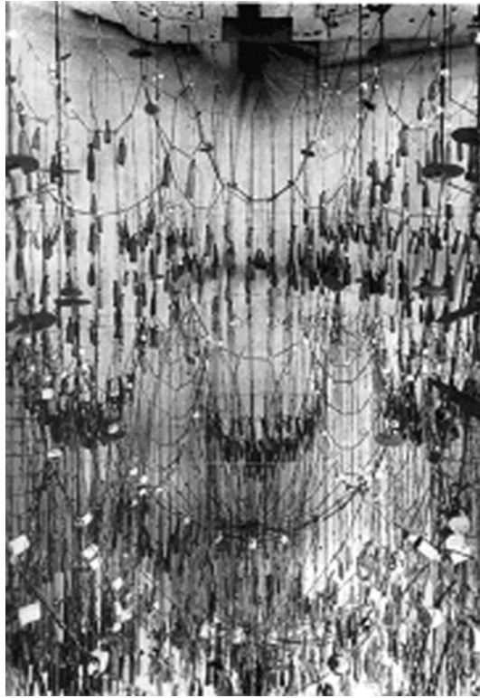
Figure 4.2.13. Funicular shapes in practice. Catalan architect Antonio Gaudi (1852–1926) used tension nets and weights to determine the funicular arch shapes for the Sagrada Familia in Barcelona.
