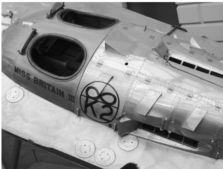
Figure 3.6.2. Miss Britain III, one time fastest boat in the world, clad in aluminum.
