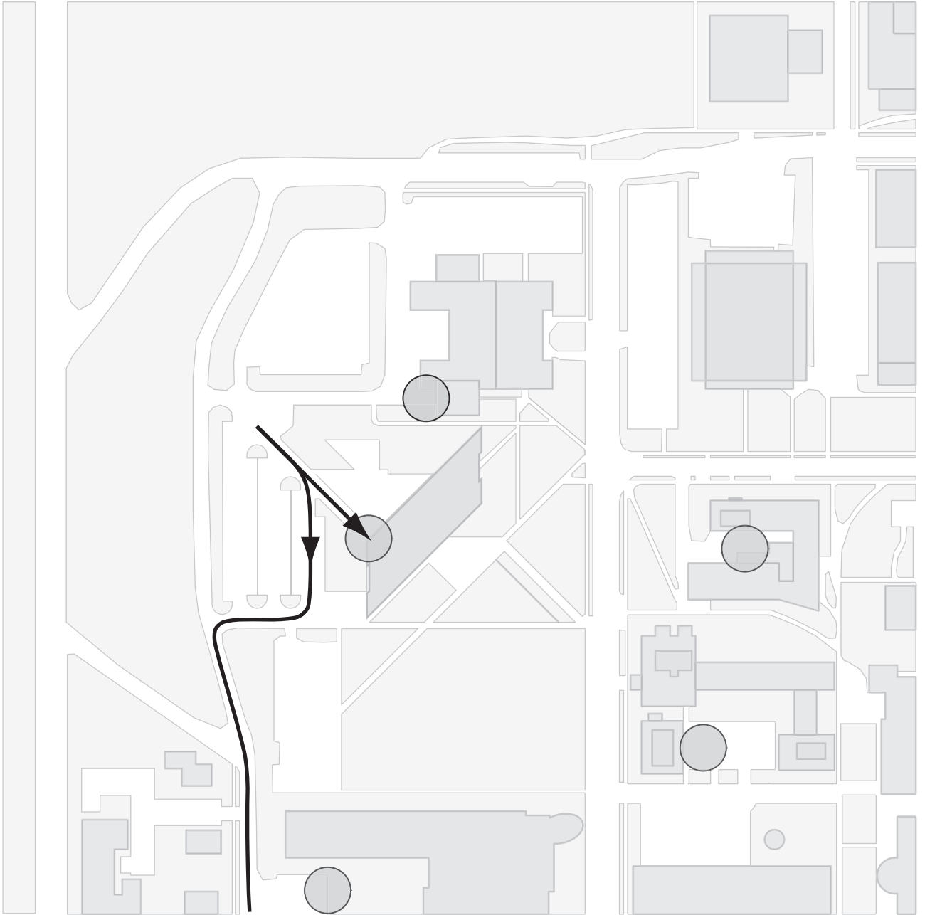
Figure 1.2.7. In addition to pedestrian and vehicular circulation, service access is an important aspect of siting and program layout. Here, the analysis notes a somewhat difficult truck access, and compares it with other, nearby service areas and truck docks.
